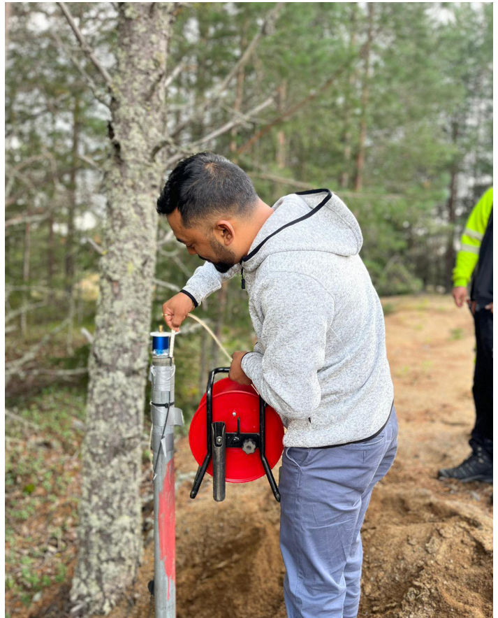
Engineer Sunil Shrestha measuring ground water levels.
